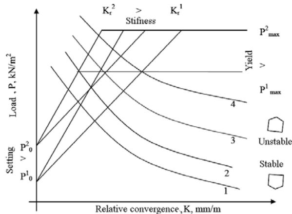
Fig. 13. Ground response curves conceptual model
