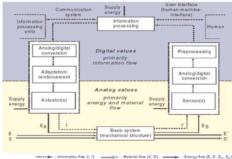
**Fig. 22.** Basic structure of a mechatronic system based on a control loop comprising basic system, sensors, information processing and actuators
