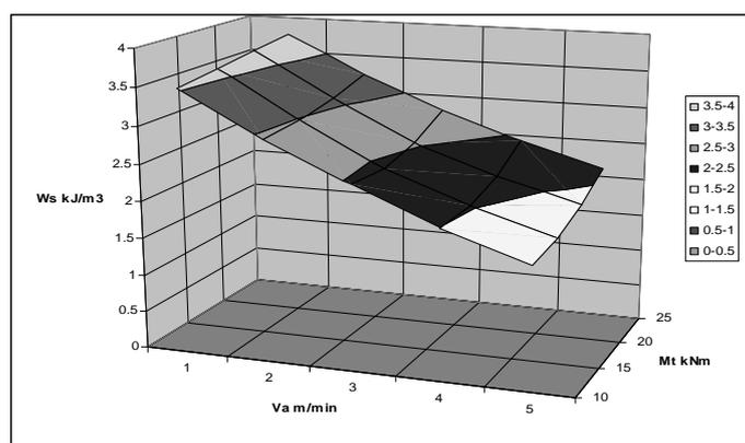
**Fig. 12.** Dependency of  $E_s$  ( $M_t, v_a$ ) for  $F_a = 700$  kN
