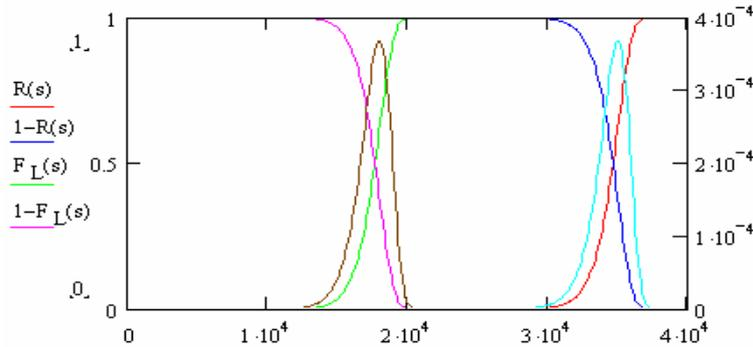
**Fig. 9.** The L-S interference charts for the excavator working in overburden rock (Specific energy consumption in 10<sup>5</sup> kWh/m<sup>3</sup> on x axis)
