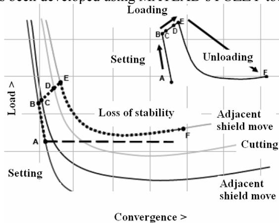
Fig. 14. Ground response curves conceptual model according to [7].
