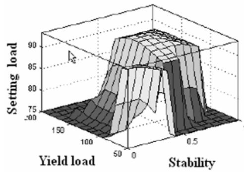
Fig. 18. Setting load as a function of stability and yield load
