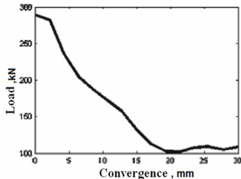
Fig. 16. Load-convergence curve of the roof
