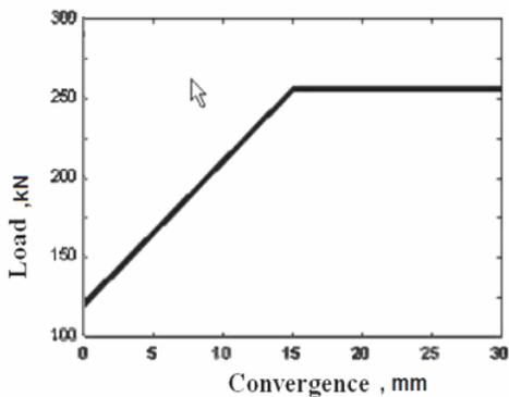
Fig. 15. Load-convergence curve of the support
