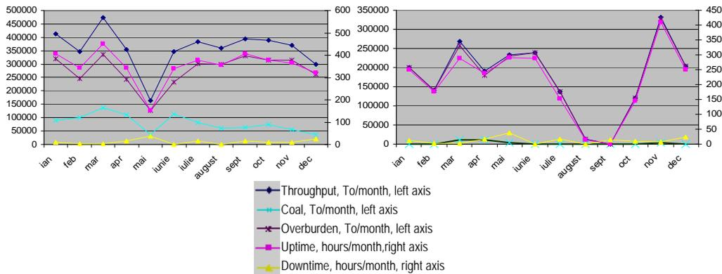
**Fig. 1.** Operation diagram of the Excavator no. 1
