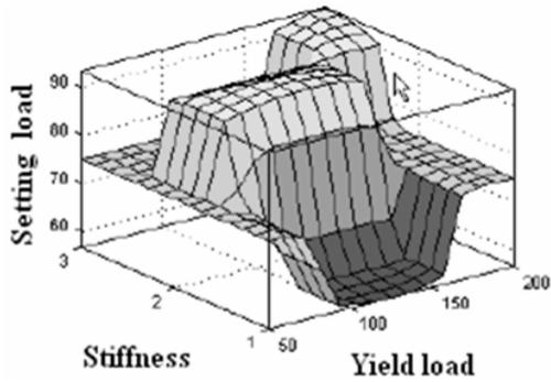
Fig. 17. Setting load as a function of stiffness and yield
