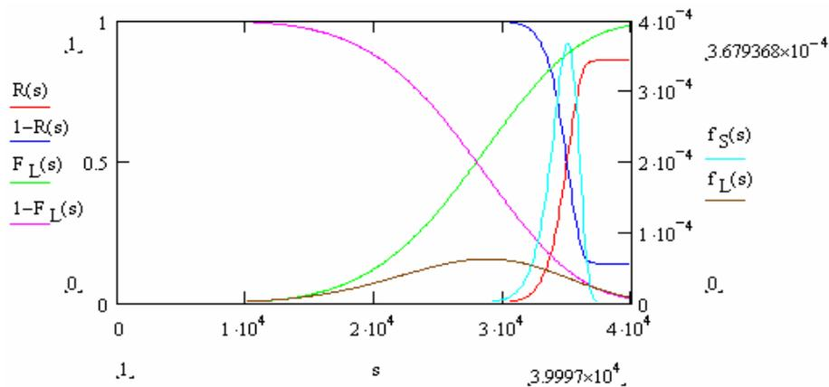
**Fig. 10.** The L-S interference charts for the excavator working in lignite (Specific energy consumption in  $10^5$  kWh/m<sup>3</sup> on x axis)
