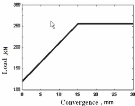
Fig. 15. Load-convergence curve of the support
